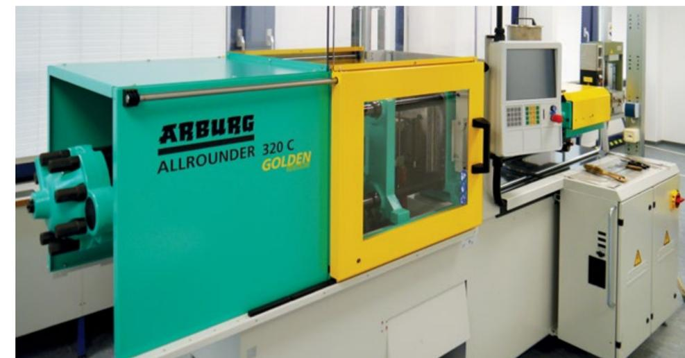
A modern injection moulding machine with a closing force of 500 kN is available for customer testing.
