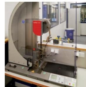
Impact pendulum operating according to the Charpy method.
